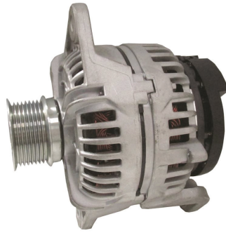
OE NO. 0124655008 RGT 1277 ALT ALTERNATOR 24V 110A NCB2 VOLVO B12B/FH12
